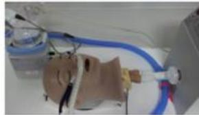
Figure 2: Respirable Dose test setup.
